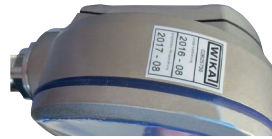
Fig. 4 - CPG1200 without protective case cap
